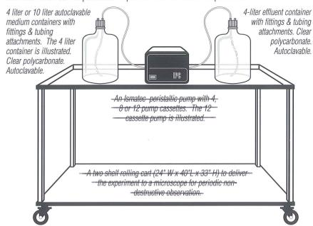
Each flow cell has three separate growth channels and each channel requires a single pump cassette to supply culture medium to it. The Stovall cart is designed to accommodate a maximum of 4 flow cells (I.E.: 12 growth channels) for a single experiment.
